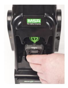
1. Insert the bottom of the instrument into the cradle and push the top until it snaps into place.
