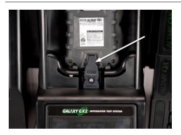
If using the charging option on the ALTAIR 4/4X instrument ensure the Test Stand charging connector at the bottom of the cradle makes contact with the instrument contact.
