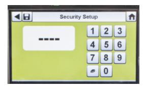
If no password is desired, enter "0000" to disable the password feature. The Test Stand is shipped with the password disabled.
