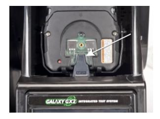
1. Insert the instrument into the cradle, sliding the bottom over the charging connector.
