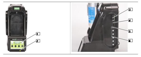
Figure 3 Test Stand Physical Features
