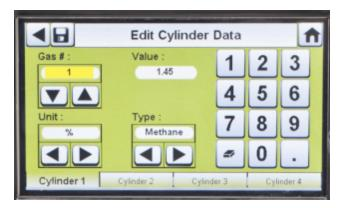
4. Set the **Gas #** by selecting either the **up or down arrows**. If there is one gas in the cylinder, select 1. **For additional gases in the same cylinder (gases 2-6)**, enter the gas parameters.
