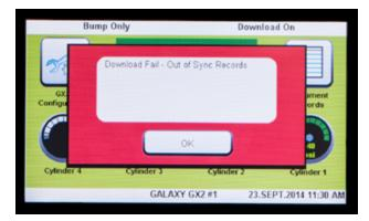
If the Out of Sync Records error is received on the test stand, see the "Out of Sync White Paper" located on the GALAXY GX2 product page on www.MSAsafety.com.
