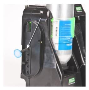
5. If not using MSA Cylinder Holders, the left most **Test Stand** should have a fresh air filter -attached to the top port.
